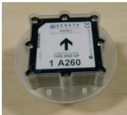
Magnetometer used as part of SCOOT installation
